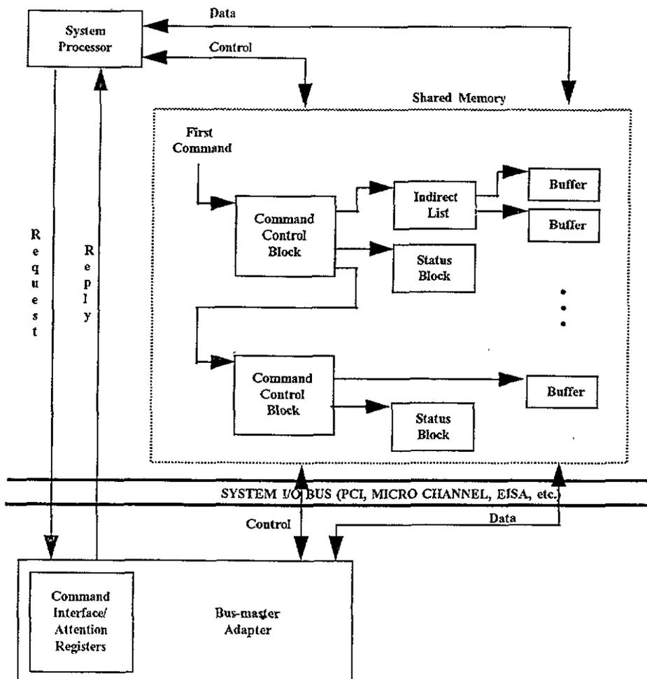
Figure 1. An interrupt-driven I/O architecture (SCB Locate Mode).
