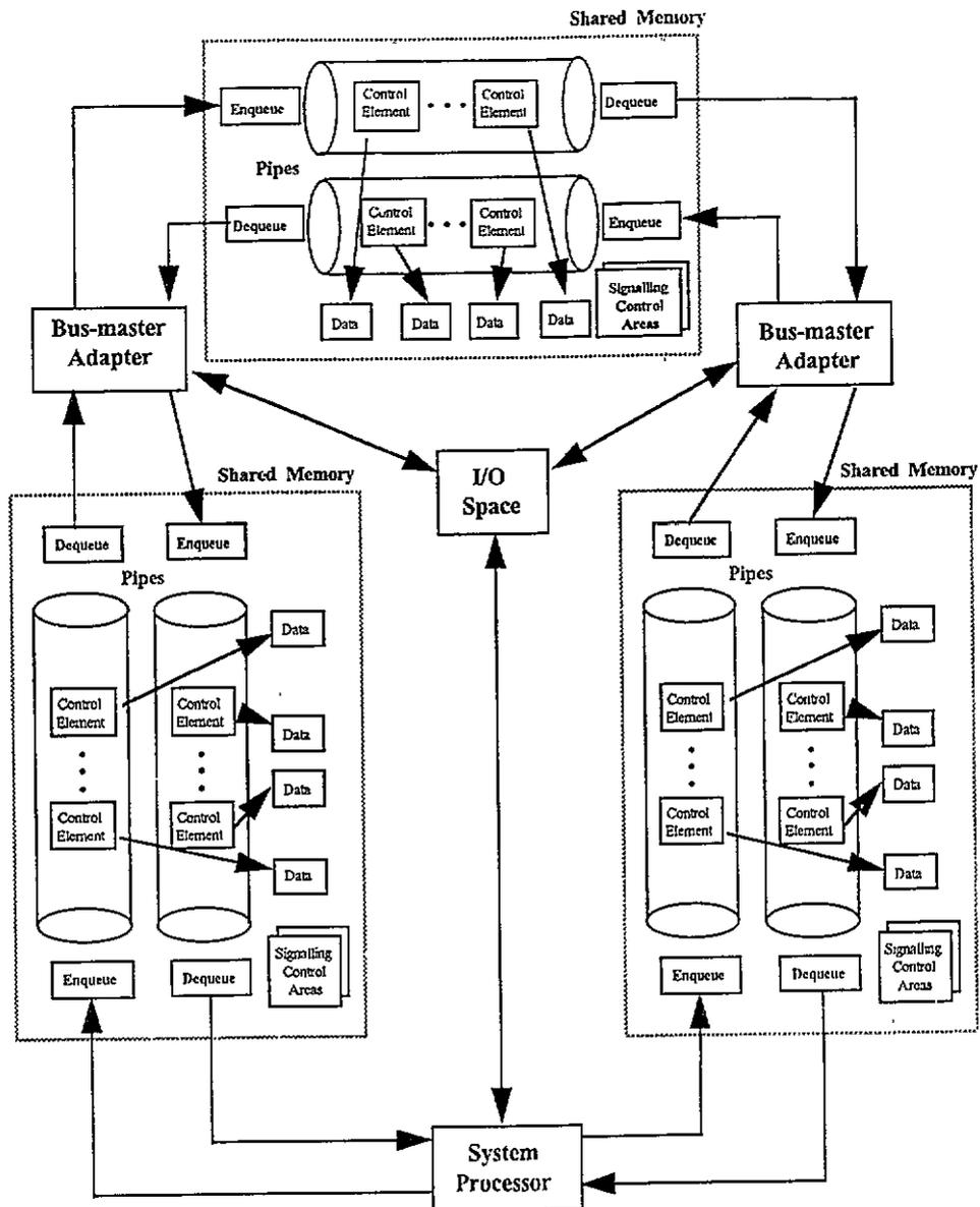
Figure 2. A peer-to-peer I/O architecture (SCB Move Mode).
