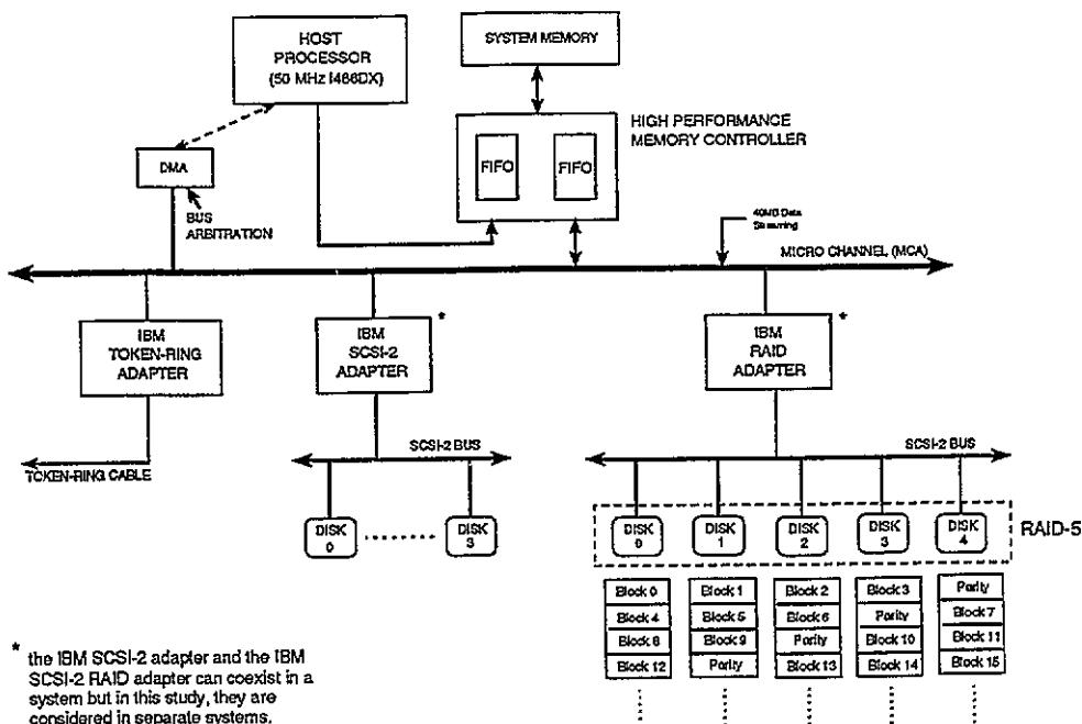
Figure 3. The IBM PS/2 Model 95 50 MHz Server.
